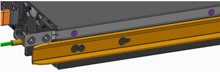
Figure 18. GND Lug/Bracket Assembly Attached to the System
